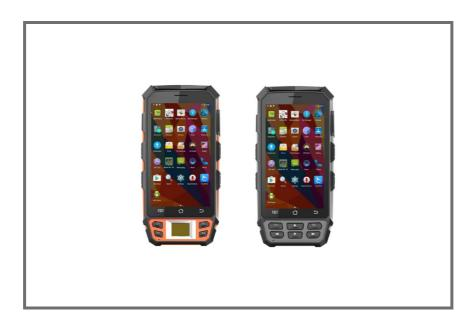
Ci-RH272 is an industrial android mobile data terminal with high integration of iot functions. The build-in 2.4Ghz active rfid reading distance reach around 50meters in open area, it is widely used for asset tracking, intelligent transportation, production line management, personnel tracking etc.
