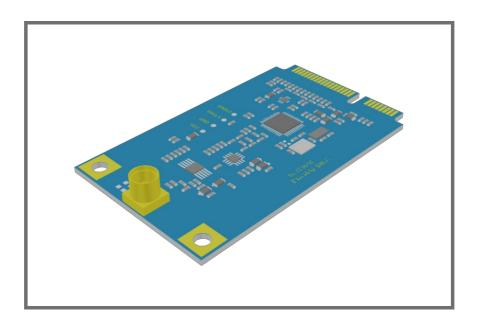
Ci-RM253 PCIE connector active RFID module operates in 2.4Ghz ISM band, it is featured with high reading speed, flexible expansion, reliable data transmission, reading range can reach around 100meters. It is mainly embedded into industrial device for data capturing, sensor data acquisition and other system integration applications.
