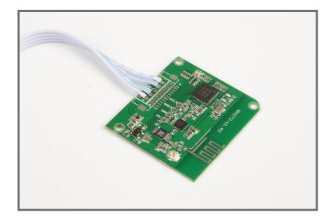
Ci-RM272 active RFID module operates in 2.4Ghz ISM band, it is very small in size with high reading speed, flexible expansion, reliable data transmission, reading range can reach around 100meters. It is mainly embedded into other device like mobile data terminal for data capturing, sensor data acquisition and other system integration applications.
